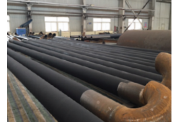
HiE-Coat™ 840-M coats gas-fired heating tubes.
