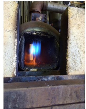
HiE-Coat™ 840-CX applied to a gas-fired forge.
