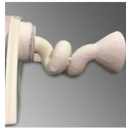
Ceramabond™ 503 coats spiral cantilevered sensor.
