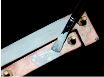
Cerabond™ 571 coats copper induction heater.
