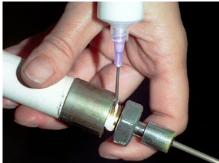
Cerabond™ 671 used as a high temp threadlocker.
