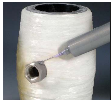
Pyro-Putty® 2400 seals high temp threads.
